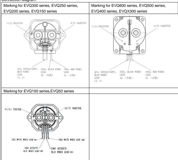
For EVQ600 series, EVQ500 series, EVQ400 series, EVQX300 series, EVQ300 series, EVQ250 series, EVQ200 series, EVQ150 series: A1 (Red wire +) and A2 (black wire -) are coil terminals. 1/L1 and 2/T1 are for main cotact terminals. .3 and .4 are for auxiliary contact terminal.
