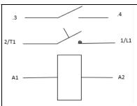
For EVQ600 series, EVQ500 series, EVQ400 series, EVQX300 series, EVQ300 series, EVQ250 series, EVQ250 series, EVQ250 series, EVQ150 series: A1 (Red wire +) and A2 (black wire -) are coil terminals. 1/L1 and 2/T1 are for main cotact terminals. .3 and .4 are for auxiliary contact terminal.
